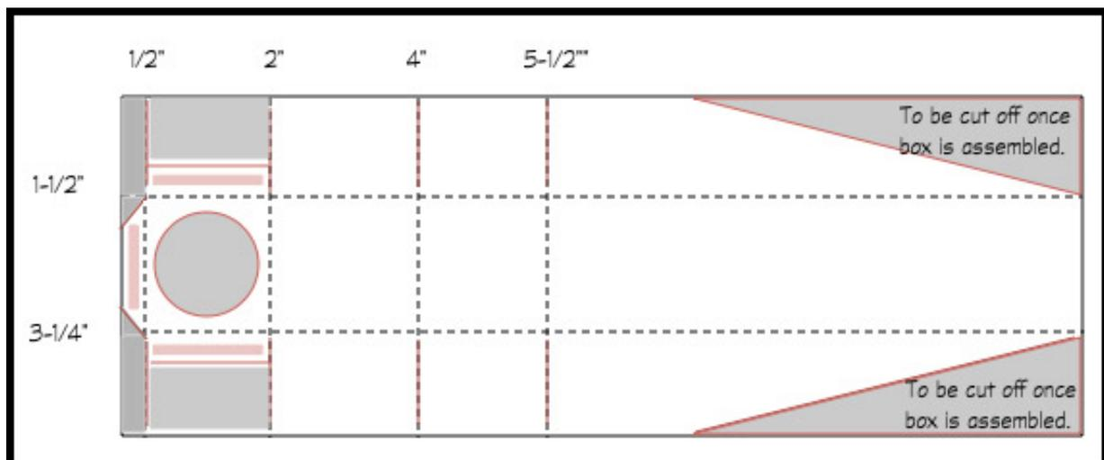
6. Cut off the 1/2" tab areas as indicated in gray. Cut a slight angle on each side of the front tab.
